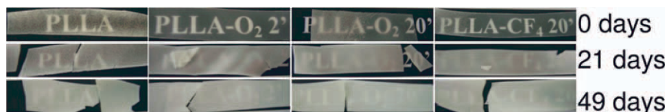
Figure 5 Photograph of pristine and treated PLLA films before and after 21 and 49 days of in vitro degradation. [Color figure can be viewed in the online issue, which is available at wileyonlinelibrary.com .]
